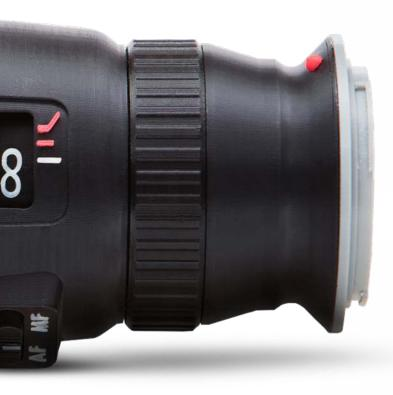
A fully functional lens prototype printed on the Zortrax M200 using Z-ULTRAT and Z-GLASS.
